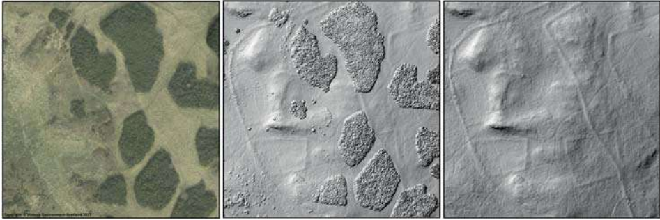
Figure 5. Aerial photography and ALS survey data for Whinny Hill, showing the DTM in the middle image and DSM, with vegetation cover 'removed' on the right. © Historic Environment Scotland
