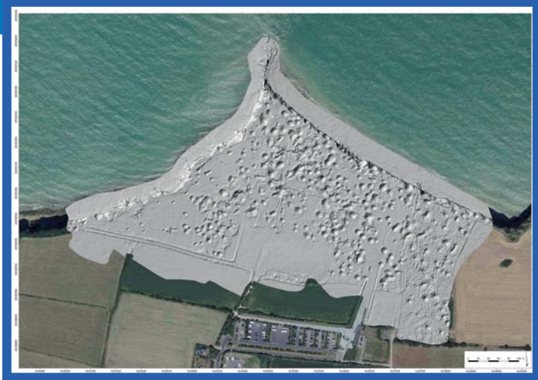
Pointe du Hoc, Calvados, Normandy. Actualised map of the battery and US Rangers' Memorial, made by INRAP after LiDAR and geophysical surveys, showing every concrete and earth feature as well as bomb craters (© V. Carpentier, INRAP)
