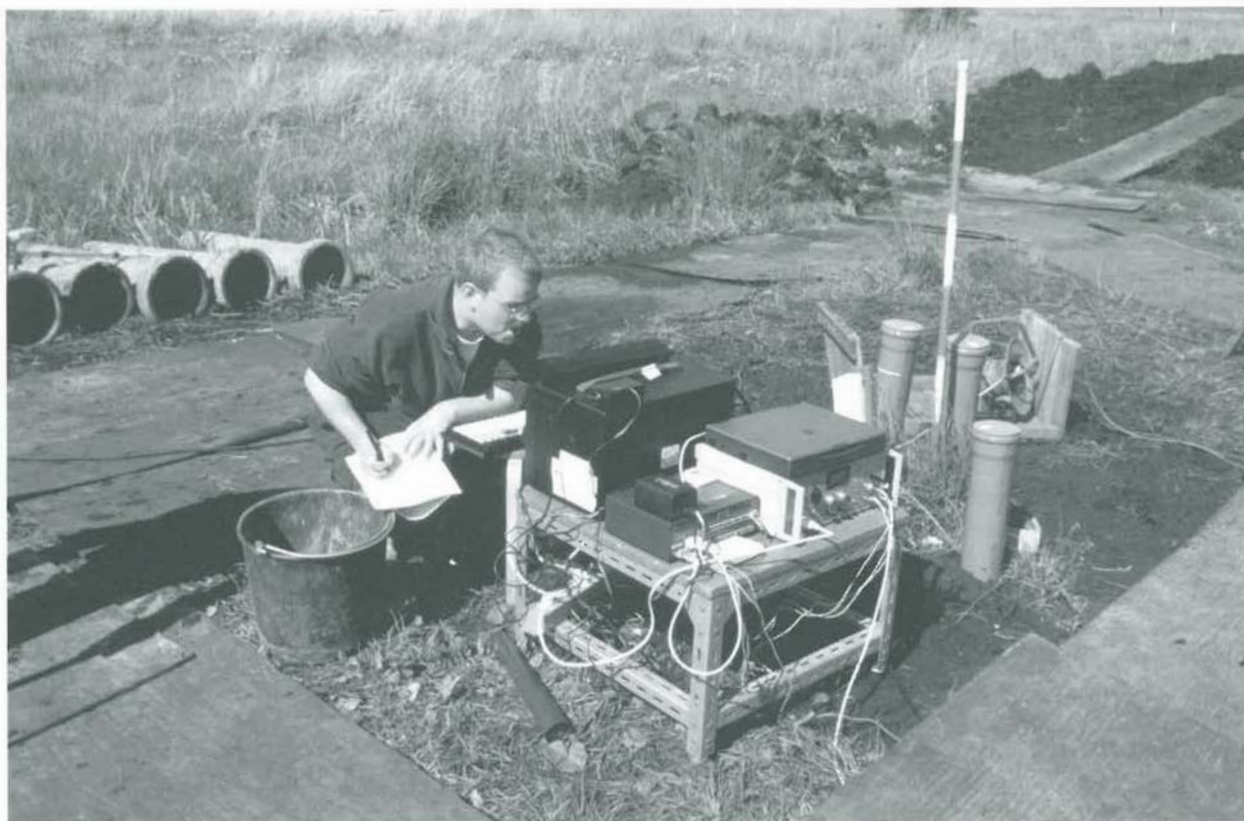
Fig.6.3: Measuring environmental parameters (oxygen and corrosion rate) relevant to the in situ preservation of buried items of wood, iron, etc. at the Iron Age votive site of Nydam. Photo National Museum of Denmark.
