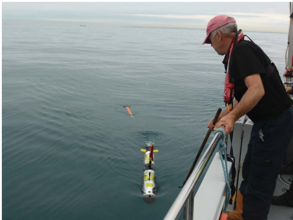
Figure 1. An Ocean Server Iver3 Autonomous Underwater Vehicle, used for underwater remote sensing (Wessex Archaeology for Historic England).
