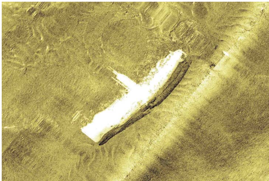
Figure 2. Sidescan sonar image of U-8 collected by an Autonomous Underwater Vehicle (Wessex Archaeology for Historic England).
