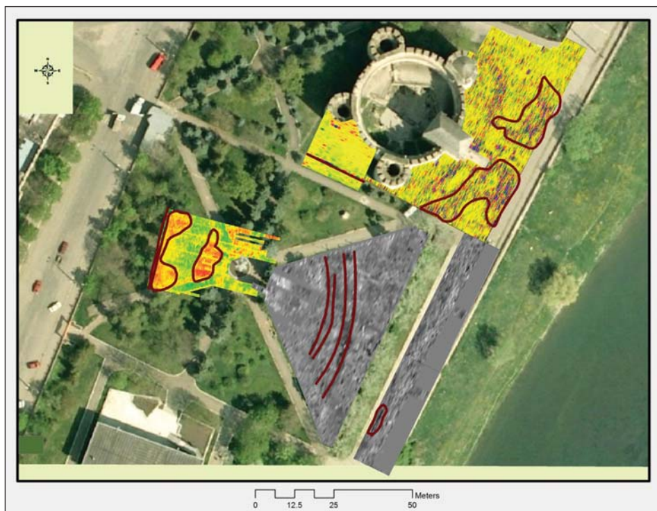
Figure 3. Soroca – medieval fortress, picture of the GPR survey (after Asandulesei et al. 2015).
