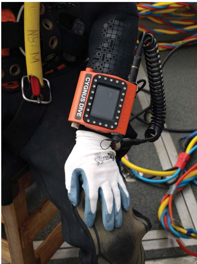
Figure 3. Cygnus DIVE underwater ultrasonic thickness gauge, used for non-destructive thickness testing (Wessex Archaeology for Historic England).
